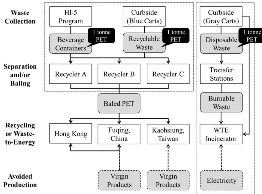
**Fig. 1.** Domestic and transboundary flows of 1 tonne of post-consumer PET bottles generated in Oahu, Hawai'i (i.e., functional unit of the study) as well as their avoided production processes. Solid and compound lines represent the flows for transboundary recycling and for energy recovery, respectively. Dotted boxes denote the system boundary of Honolulu, Hawai'i.
