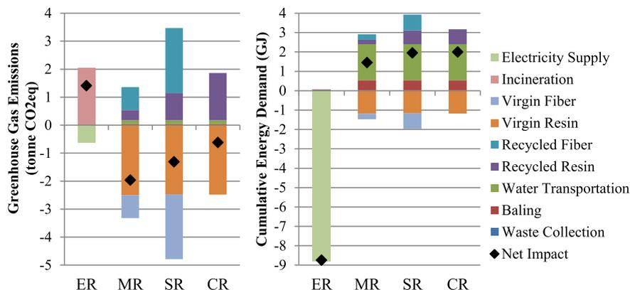
Fig. 2. Greenhouse gas emissions (left) and cumulative energy demand (right) of the four evaluated scenarios: ER (Energy Recovery), MR (Mechanical Recycling), SR (Semi-mechanical Recycling), and CR (Chemical Recycling).
